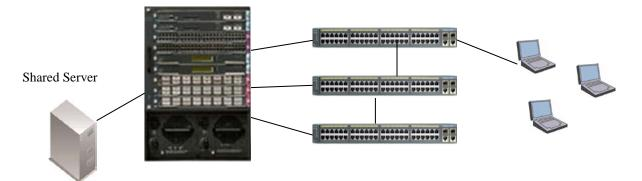
OSPF uses an algorithm that selects the shortest open path between routers. The laptop users above are in different IP subnets, each with different IP addresses. In order to communicate with shared resources (i.e. printers/servers) as well as the WAN via the core router, Layer 3 routes must be established. OSPF will determine the best, fastest route to those resources. Each OSPF router maintains routing tables of all other OSPF routers for best route determination.
